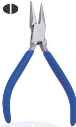
Ai-787 Chain Nose Pliers 130mm Smooth Stainless Steel Made, Box Joint without Leaf Spring, Satin Finish Pvc Handles.
