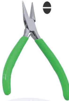
Ai-805 Chain Nose Pliers 115mm Stainless Steel Made, Box Joint with Double Leaf Spring Satin Finish, Pvc Handles.
