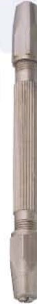
Ai-1024 Tool Holder with 2 sided reversible chucks one side holds blades and other side for round objects (clamping range 2.6mm to 3mm).
